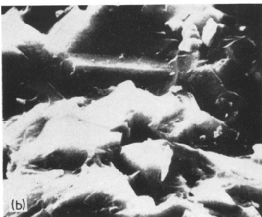
Figure 4 Scanning micrograph showing flaws at the base of a machined notch in an uncrystallized glass, \times 120 .
